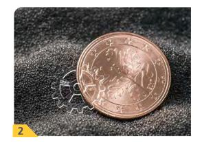
Laser-cut glass gearwheel with marking
