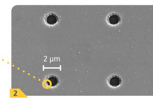
1 Micro drillings in stainless steel foil t = 30 μm with diameter < 4 μm</p> 2
