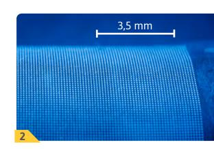
2 Laser drilled PTFE membrane, bore diameter 25 μm
