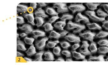
1 Roughened metal surface with geometric undercuts
