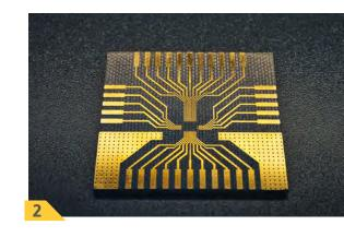
1 Isolation trenches on a metallized ceramic substrate
