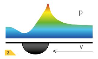
Functional diagram of hydrodynamic pressure build-up (pressure/velocity)
