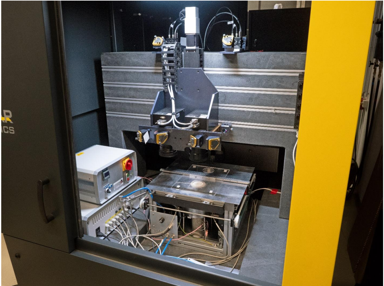
Laser machine RDX1000 for selective laser sintering (SLS) for the production of porous glass moldings developed within the scope of "LASERPORE" (Source: EAH Jena)
