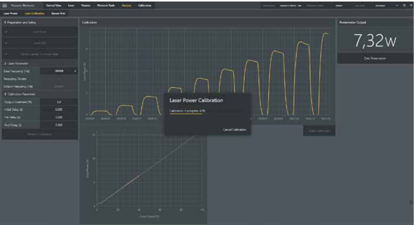
Continuous calibration of the laser power: A calibration curve is created for a specific set of parameters and stored in the database
