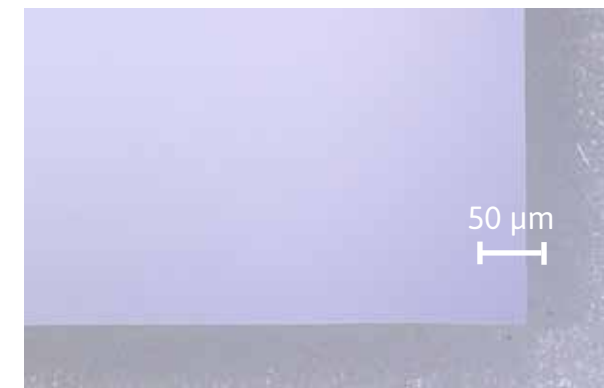
Angular contour cut in \text{Al}_2\text{O}_3 with edge radius < 10 µm
