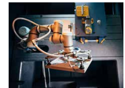
The machine bed of the plant is made of natural stone. To be seen on the picture: Robotic insert in the RDX800
