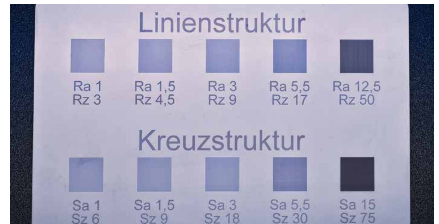
Generation of defined Ra/Sa values in ceramics
