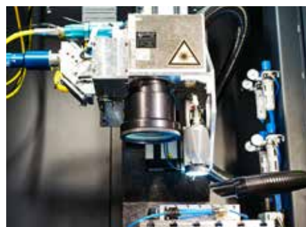
Interior view of the RDX2Fiber with precise axis system, galvanometer scanning system and measurement technology
