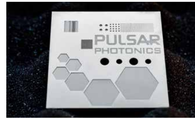
Structuring examples in an \text{Al}_2\text{O}_3 -ceramic
