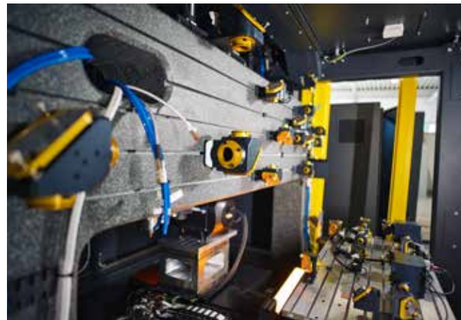
Interior view of the RDX800 during an assembly of the beam delivery systems
