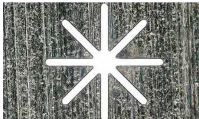
Star-shaped microcuts in stainless steel
