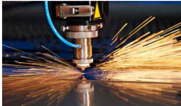
Melt dominant QCW drilling process
