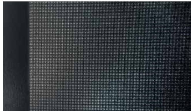
Laser micro-holes in a tungsten foil
