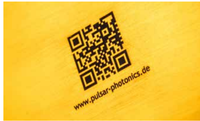
Resistant laser marking in steel surface
