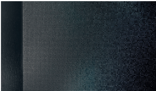
Laser micro-holes in a tungsten foil
