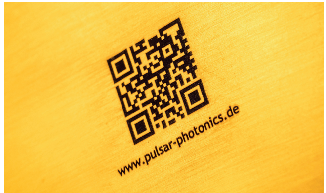
Resistant laser marking in steel surface
