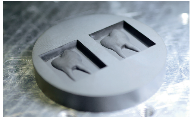
2.5D Structuring: Root of a dental implant made of a high-performance ceramic material
