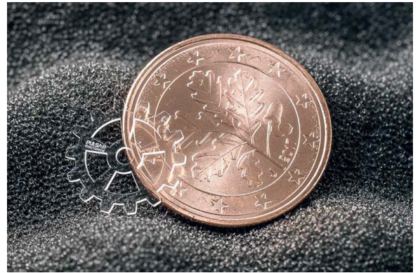
Laser precision cut glass gear with marking
