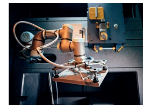
The machine bed of the plant is made of natural stone. To be seen on the picture: Robotic insert in the RDX800
