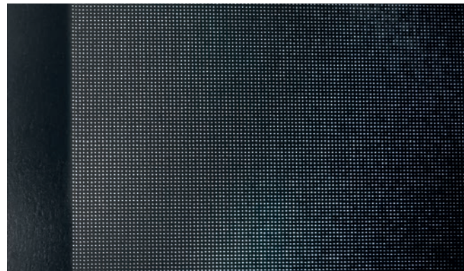
Laser micro-holes in a tungsten foil
