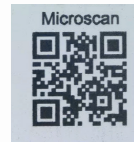
High resolution QR code with dimensions 300 \mu\text{m} x 300 \mu\text{m}
