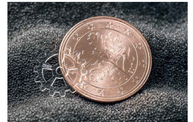
Laser precision cut glass gear with marking
