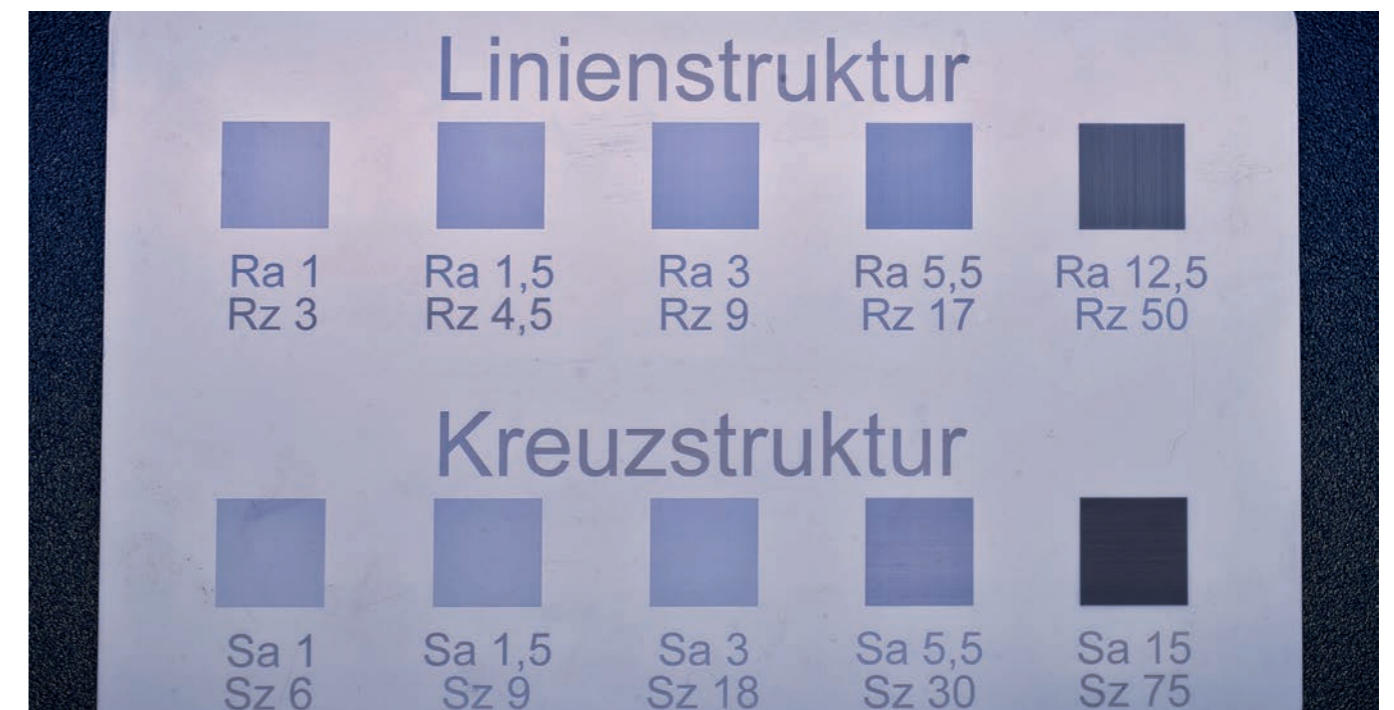
Generation of defined Ra/Sa values in ceramics
