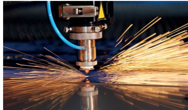
Melt dominant QCW drilling process
