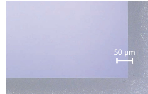
Angular contour cut in \text{Al}_2\text{O}_3 with edge radius < 10 \mu\text{m}
